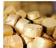
Casting billets are extruded in the extrusion workshop. To follow, the sizing, cutting, tension and anti-wobbling operations are done according to the produced cross-section. These products are delivered to the customers after being packed.
